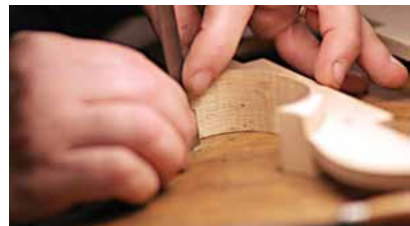
Above, from left: Master luthier James Banicki carves a violin's back plate. Crafting a violin requires delicacy and detail. Carving an inlay channel and setting in ribbing. Left: A violin hand-crafted in the Vermont Violins workshop, antiqued in the traditional Italian style.
