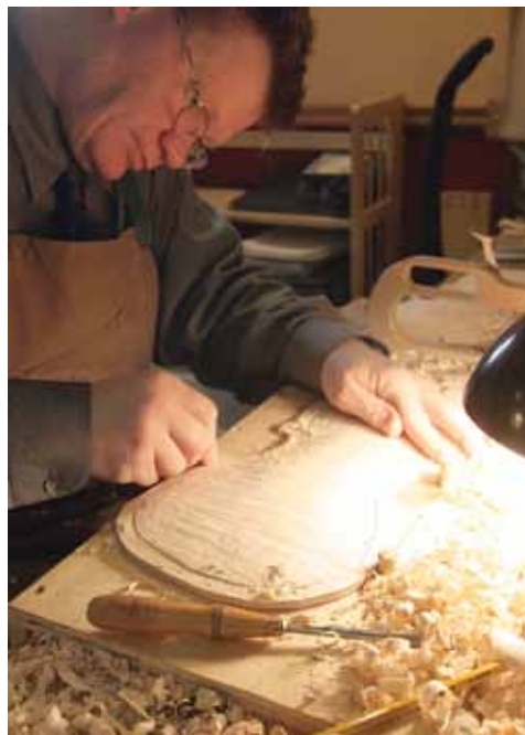
Above, from left: Master luthier James Banicki carves a violin's back plate. Crafting a violin requires delicacy and detail. Carving an inlay channel and setting in ribbing. Left: A violin hand-crafted in the Vermont Violins workshop, antiqued in the traditional Italian style.
