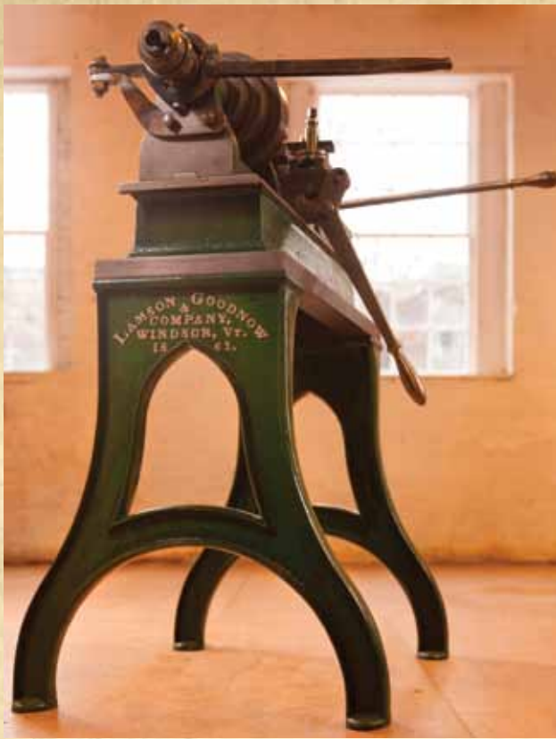
Above: Rifling Machine, Robbins & Lawrence, Windsor, Vermont, 1853. In the 1850s, machine designers, including those in Windsor, developed power machines for cutting the grooves at a predetermined depth and angle. Powered by the overhead line shaft and driven by a waterwheel, the rifling machine worked all day without tiring. Photo by First Light Studio. Right: Robbins & Lawrence Armory, 1846, a National Historic Landmark, beside the Mill Brook. Photo by Jack Rowell. Below, from left: Equipment on display. Photo by Jack Rowell. William Munson's spurs and powder flask. Photos by First Light Studio.
