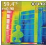
Infrared Thermal Imaging shows no insulation in the cold (blue) wall.
